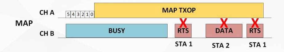
MAP fails to receive on Channel B during an ongoing frame exchange on Channel A
